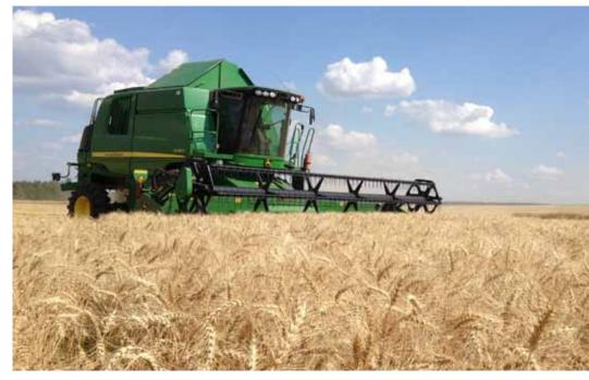
"The Balzer system makes it unnecessary to stop the combine during grain unloading," says Nikolai Lavrentev. "Thus, the productivity of four grain harvesters has grown by 30%."
