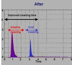
Example before and after optimization: the peaks are higher and narrower, meaning that alkaline and acid cleaning is done more effectively and in a shorter time span resulting in substantial cost and time savings.
