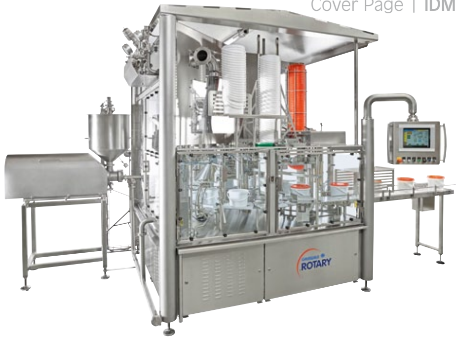
The new format independent rotary-type bucket filler GRUNWALD-ROTARY XL (photo: GRUNWALD)
