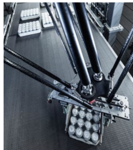
For the first time on a beverage filling line a highly dynamic handling system is being used on the KHS InnoDry Block to create precise layer patterns (photo: KHS)
