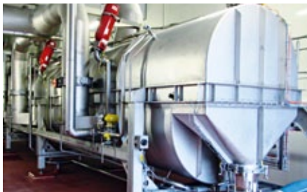
Whey 5 has two fluid bed dryers (photo: UTM)
