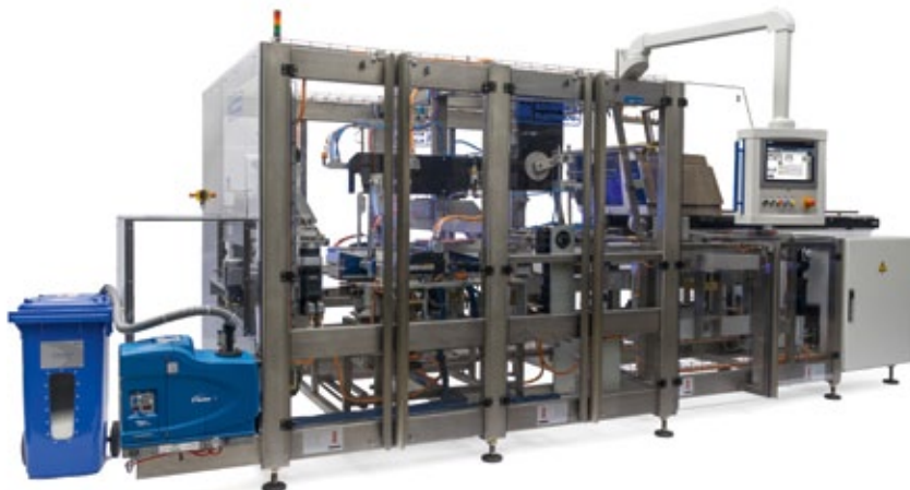
Carton Erector SFS 350 by Schäfer & Flottmann (Photo: Schäfer & Flottmann)
