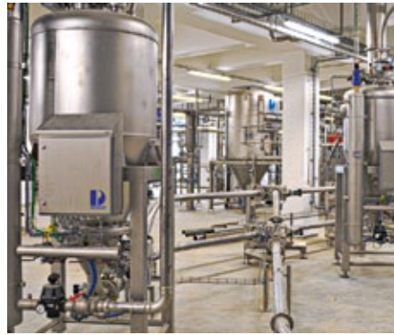
The main stream powder conveying was solved using pressure vessels (photo: Derichs)
