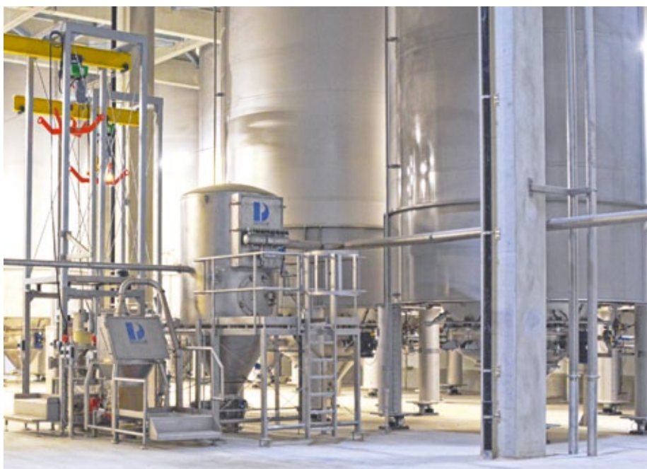
Product feed via bag discharge station and Big Bag discharge (photo: Derichs)
