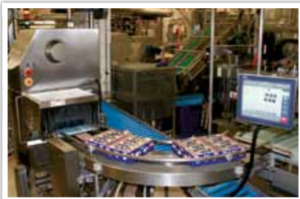
X-ray scanner SC 5000 with separate display – individually adjustable and easy to operate
