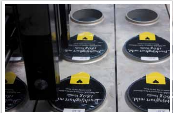
Two alphaJETs print the best-before-date "Hemme Milch means enjoying milk and delicious dairy products every day"
