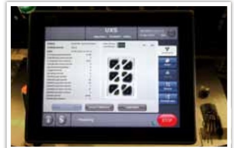
Clearly arranged display showing an X-ray of the “corner yoghurt” in its tray
