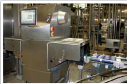
X-ray scanner SC 5000 with large conveyor body especially for yoghurt trays OCS_X-ray scanner SC 5000: At Müller, the OCS SC 5000 scanners check the famous twin pot Corner yoghurt as well as several normal single yoghurt pots
