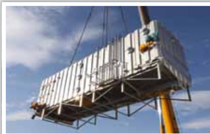
MTA - DRS curd draining belt before being installed at the customer's facility
