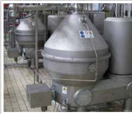
The prolong-concept by GEA Westfalia Separator Group produces milk with prolonged shelf-life with a fresh taste similar to pasteurized milk (photo: GEA Westfalia Separator Group)
