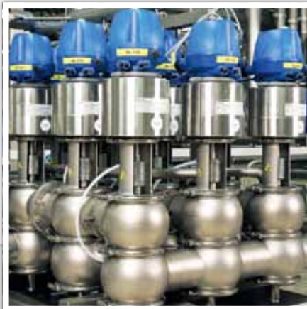
Varivent mixproof valves in a valve matrix equipped with feedback system T.VIS A8 (photo: GEA Tuchenhagen)
